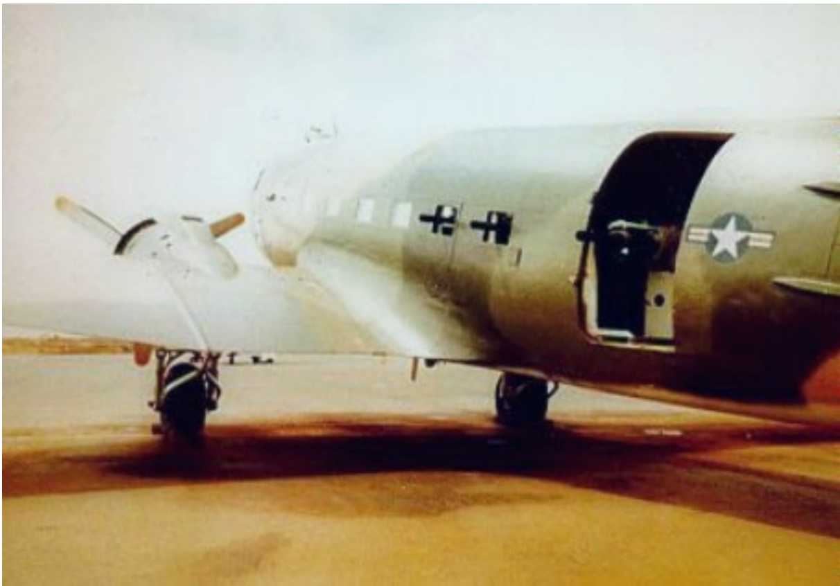
"AC-47 gunship - one Gatling gun points out the cargo door, and one each points out of the two windows forward of the door" by U.S. Air Force - National Museum of the U.S. Air Force photo 050502-F-1234P-003. Licensed under Public Domain via Commons -
